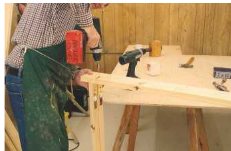
▲ Pic.14 The head, sill and pulley stiles can now be assembled and placed to one side
